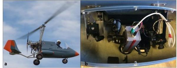
Figure 1: a) The RadGyro during a flight; b) The SOC710-GX in grey and a digital camera located in one of the two lateral compartments of the aircraft.
